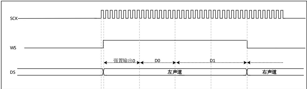
图 29-24 I2S LSB justified standard (24-bit frame, CPOL=0)
