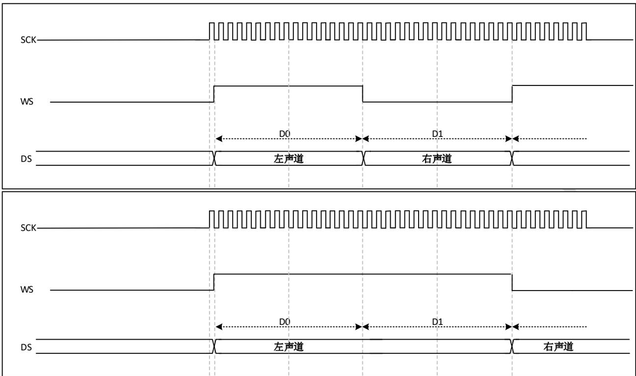
图 29-16 I2S MSB justified standard (16/32bit full accuracy, CPOL=0)
