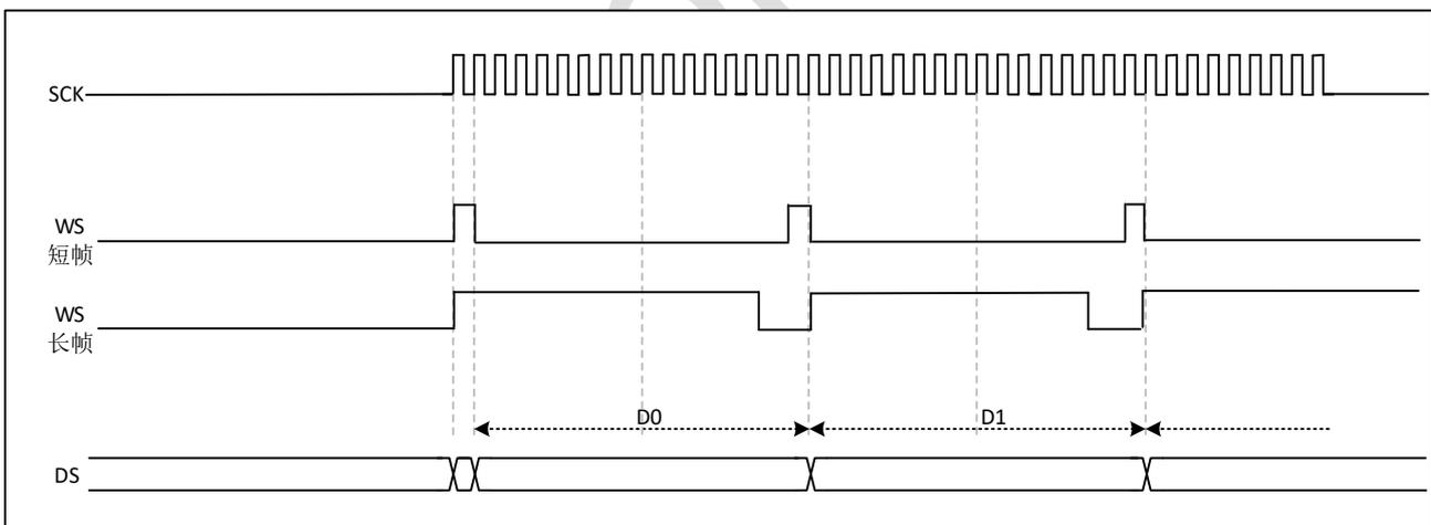
图 29-28 I2S PCM standard (16-bit frame, CPOL=0)
