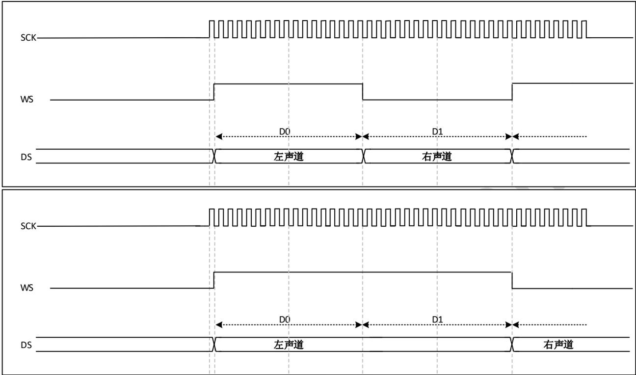
图 29-22 I2S LSB justified standard (16/32bit full accuracy, CPOL=0)
