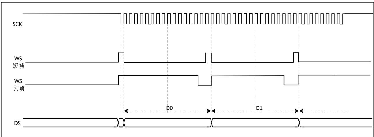
图 29-29 I2S PCM standard (16-bit frame, CPOL=1)
