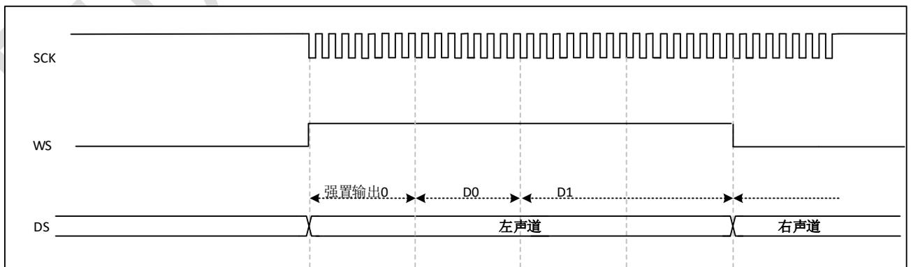
图 29-21 I2S MSB justified standard (16-bit extended 32-bit, CPOL=1)
