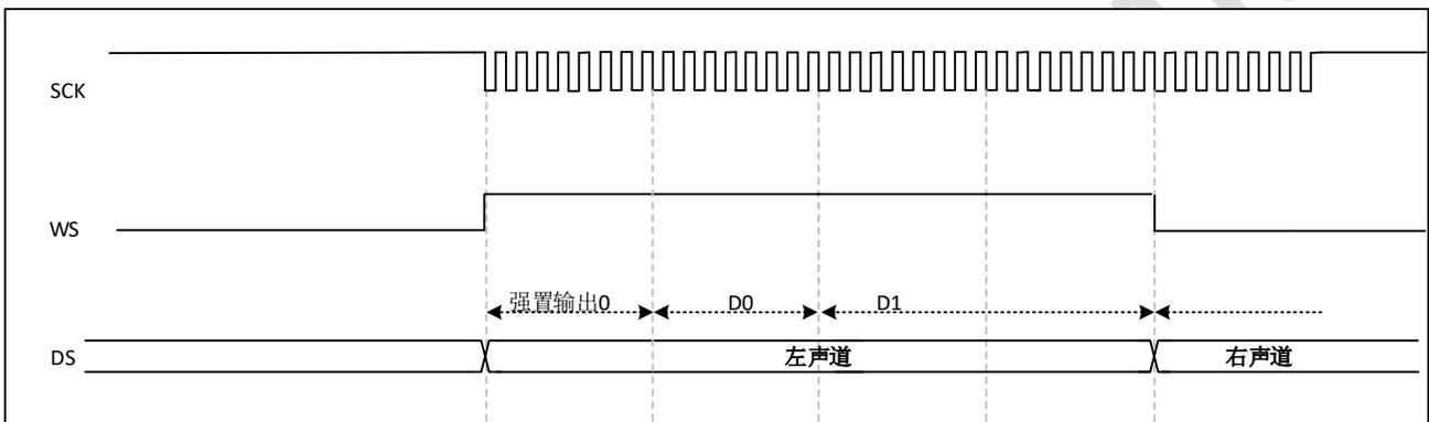
图 29-25 I2S LSB justified standard (24-bit frame, CPOL=1)
