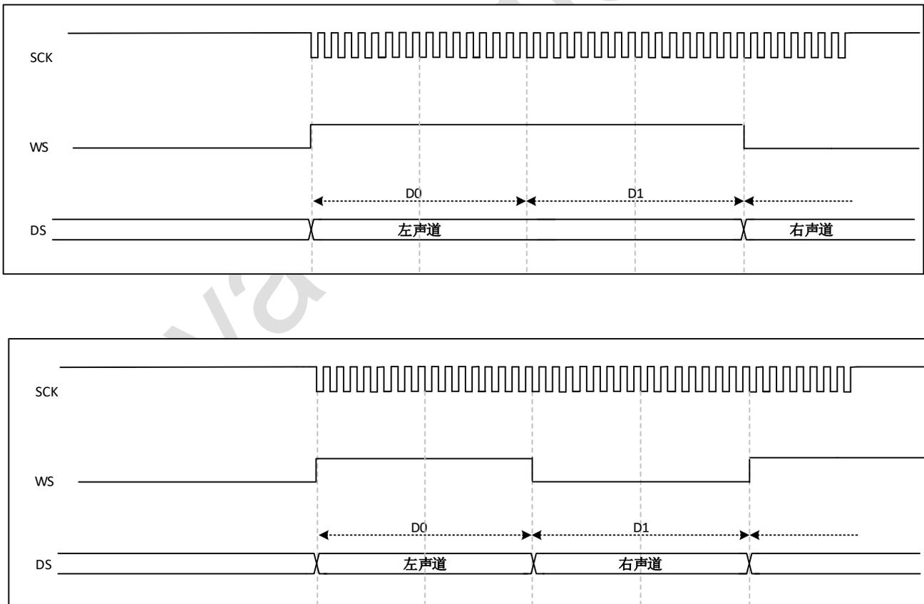
图 29-17 I2S MSB justified standard (16/32bit full accuracy, CPOL=1)
