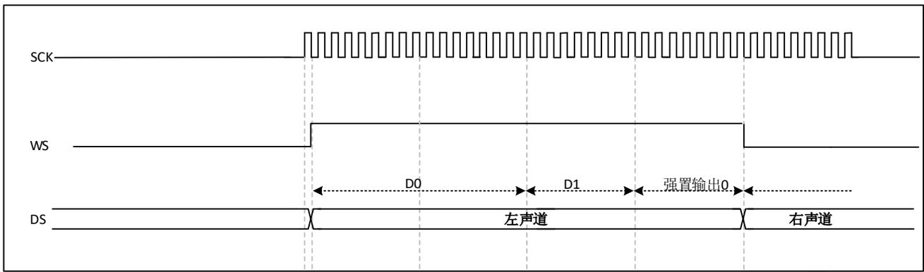
图 29-18 I2S MSB justified standard (24-bit frame, CPOL=0)
