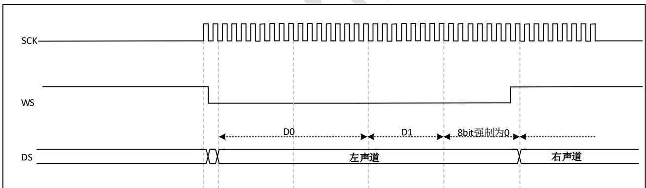
图 29-13 I2S Philips protocol (24bit frame, CPOL=0)
