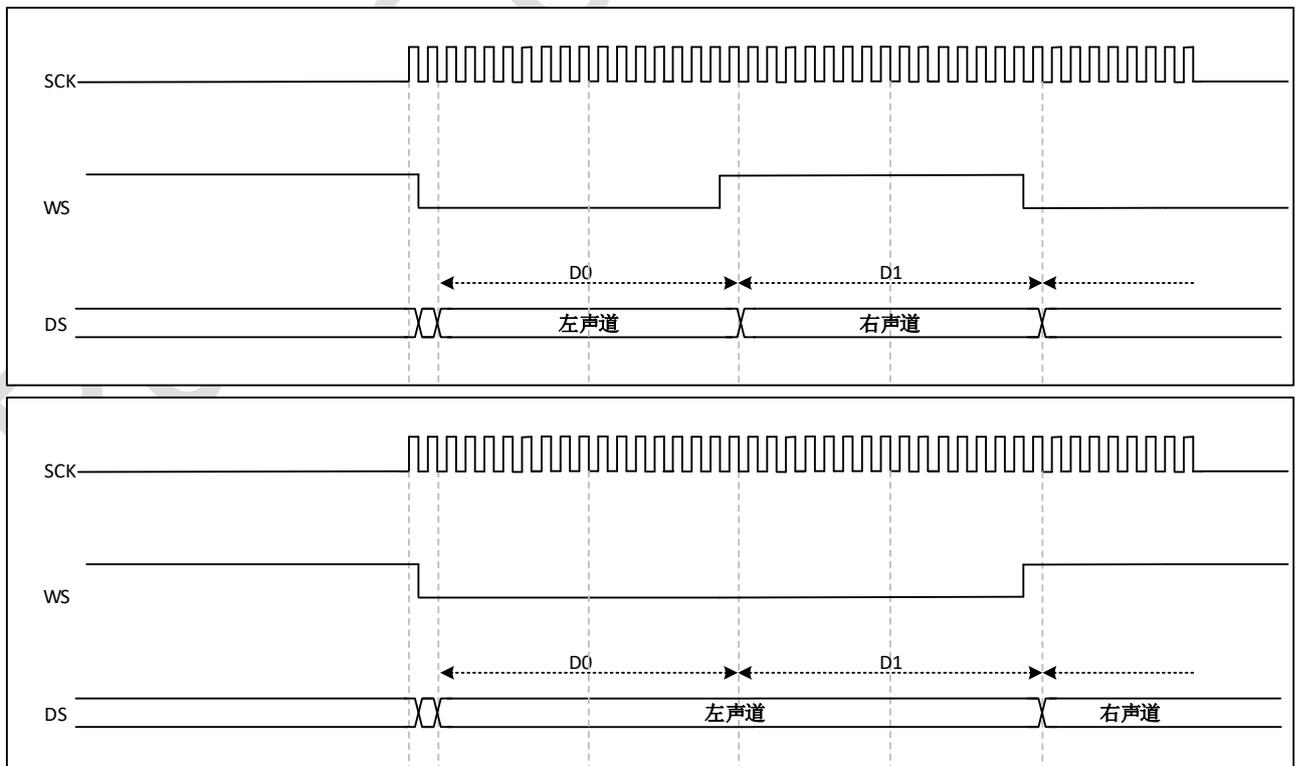
图 29-11 I2S Philips protocol (16/32bit full accuracy, CPOL=0)
