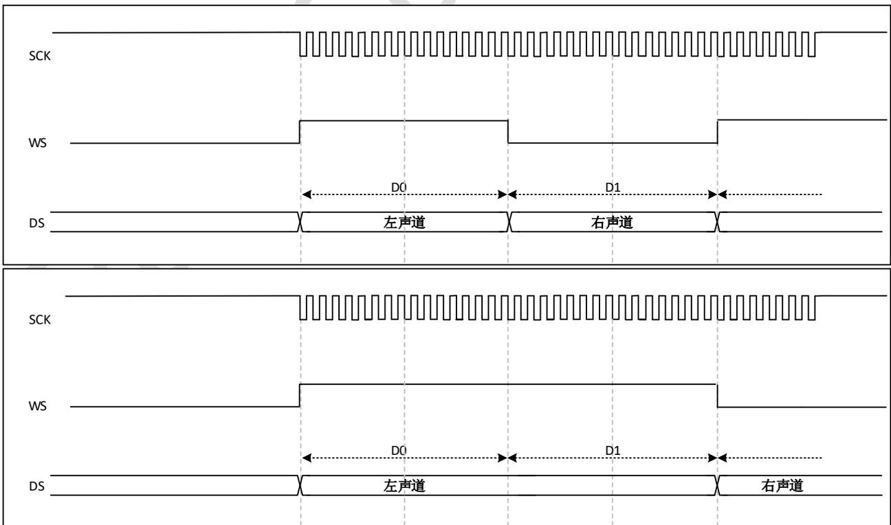
图 29-23 I2S LSB justified standard (16/32bit full accuracy, CPOL=1)
