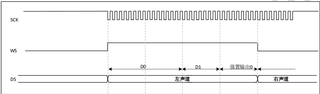
图 29-19 I2S MSB justified standard (24-bit frame, CPOL=1)
