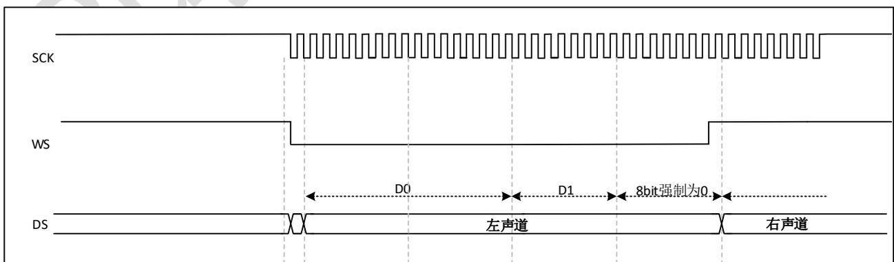
图 29-14 I2S Philips protocol (24bit frame, CPOL=1)
