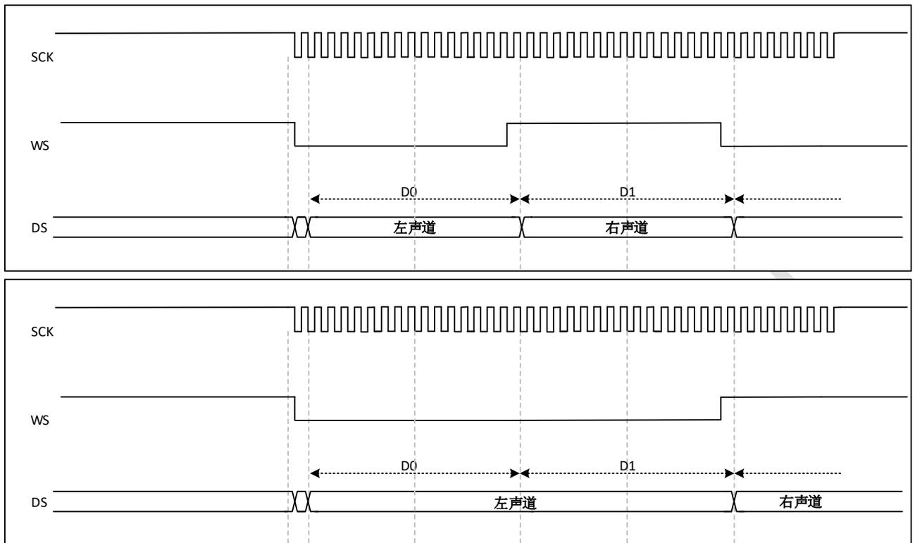
图 29-12 I2S Philips protocol (16/32bit full accuracy, CPOL=1)
