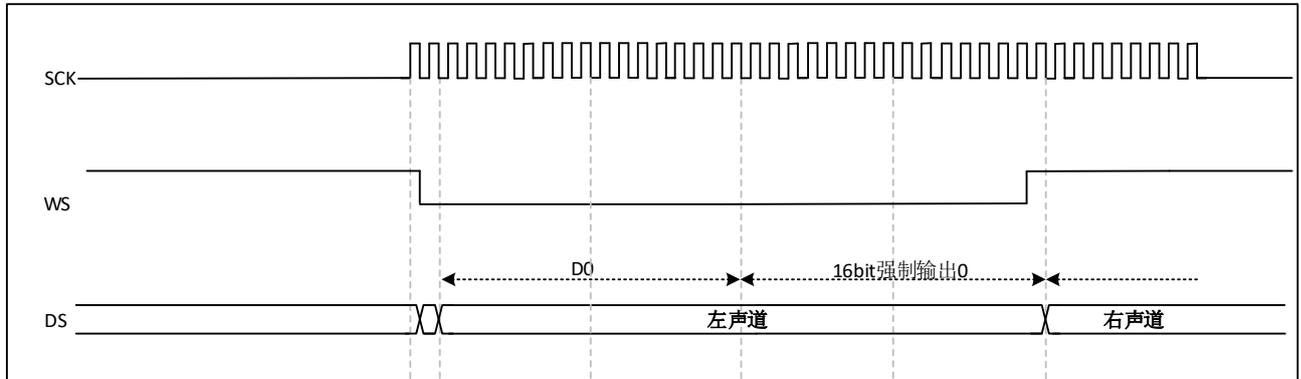
图 29-15 I2S Philips protocol (16-bit extended to 32-bit)
